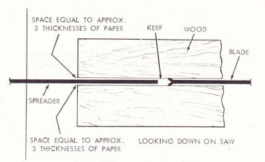
15. Make two folds in a small piece (6 x 6 in.) of ordinary NEWSPAPER making three thicknesses.
