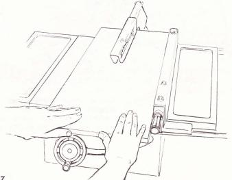
When "WIDTH OF RIP" is 2 in. to 6 in. wide USE THE PUSH STICK to feed the work.
