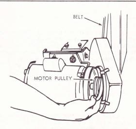
8. Press guard onto support so that bottom of guard is approximately 3/4 in. away from belt.
