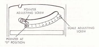
If blade is NOT SQUARE to table . . . the  $90^{\rm O}$  LIMIT STOP must be ADJUSTED.
