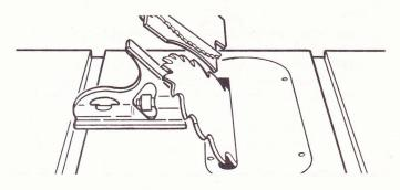
If blade is NOT  $45^{\rm o}$  to table . . . the  $45^{\rm o}$  STOP COLLAR and SCALE must be ADJUSTED.
