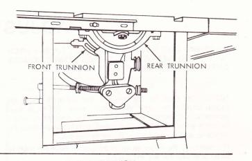
7. Loosen all three screws that hold the rear trunnion and all three screws that hold the front trunnion.
