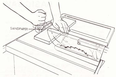
The miter gauge may be used in either of the grooves in the table. Make sure it is locked.
