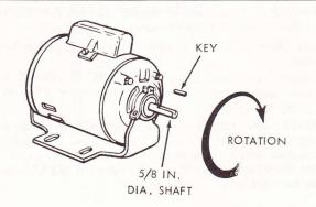
WARNING: FOR YOUR OWN SAFETY, MAKE SURE PLUG IS NOT CONNECTED TO POWER SOURCE OUTLET WHEN CHANGING MOTOR ROTATION.
