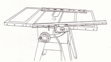
1-3/4 inch long screw through the SEVENTH hole in bar. Insert two 3/4 inch long screws through two flat washers, through holes in switch, and then through holes EIGHT and TEN in bar. Install two lockwashers and nuts then tighten.
