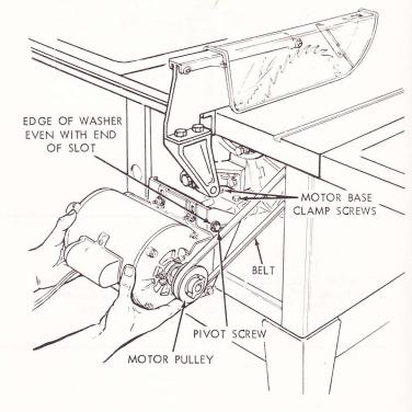
20. Loosen the two MOTOR CLAMP SCREWS on each end of motor. Rotate the motor so that the CAPACITOR COVER is on top...tighten the screws. The ventilation holes are now facing downward which will help prevent sawdust from entering motor.
