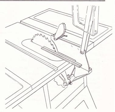
14. IMPORTANT: The SPREADER must always be PARALLEL to the sawblade and in the MIDDLE of the cut (KERF) made by the sawblade.
