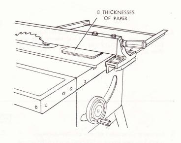
19. Move fence to RIGHT edge of table ... make sure it is approx. 1/32 in. above table at front and rear and tighten screws.
