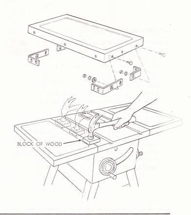
Lay REAR FENCE GUIDE BAR on table to act as a straightedge. If outer edge of extension is higher or lower than table surface;
