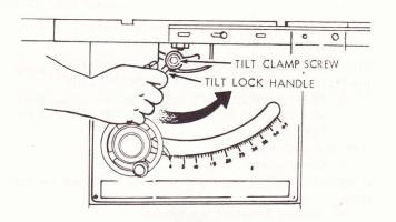
5. Rotate tilt handwheel CLOCKWISE a few turns to tilt blade. Now rotate handwheel COUNTERCLOCKWISE until it stops. Blade should now be square with table and pointer should point to "0".
