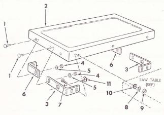
FIGURE 8 – TABLE EXTENSION SUPPLIED WITH MODEL 113.298032 AND 113.298240
