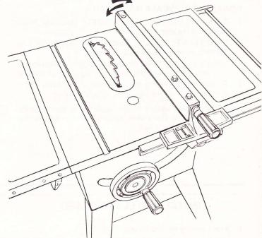
If the fence does not slide easily along the bars, the pressure of the spring can be REDUCED.
