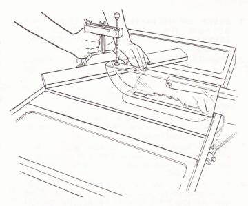
**SUPPORT LONG WORKPIECES** ... you can make a simple support by clamping a piece of plywood to a sawhorse.
