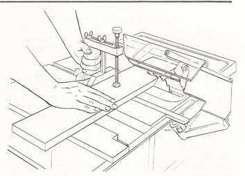
workpiece thru the sawblade. For narrow work, place other hand so thumb is hooked behind miter gauge head and fingers hooked over leading edge for work. For wider work where other hand cannot span board as above, place hand on top of work and hook fingers over leading edge of work to hold it tight against the face of the miter gauge during the cutting operation.
