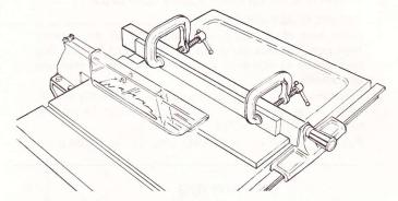
Feed the workpiece by hand along the AUXILIARY FENCE until the end is approx. 1 in. past the front edge of the table. Continue to feed using the PUSH BLOCK.
