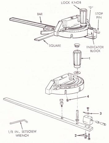
adjusted by tightening or loosening the setscrew (4) . . . using the 1/8 in. setscrew wrench.
