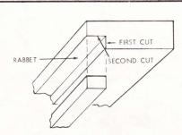
narrower make the rabbet cut with the board flat on the table using the miter gage fitted with a facing (per "6. MITER GAUGE" on p.21). DO NOT use the rip fence.
