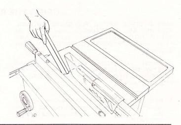
When WIDTH OF RIP is NARROWER than 2 in., the push stick CANNOT be used because the guard will interfere . . . USE the AUXILIARY FENCE/WORK SUPPORT and PUSH BLOCK.
