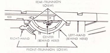
8. Using a wood block and mallet as shown, move rear trunnion to right or left as required to realign the blade. If necessary, shift front trunnion in similar manner; but do NOT move front trunnion unless necessary. Recheck the alignment with the square, then securely retighten all six trunnion screws.
