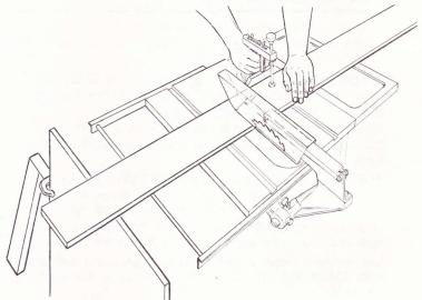
Always release clamping knob — unclamp workpiece and disengage clamp lock latch before pressing in rapid approach button.
