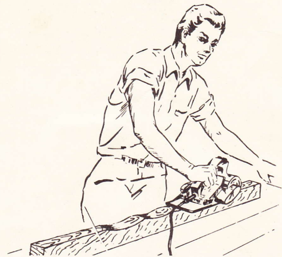
Cut resulting from improperly aligned base
